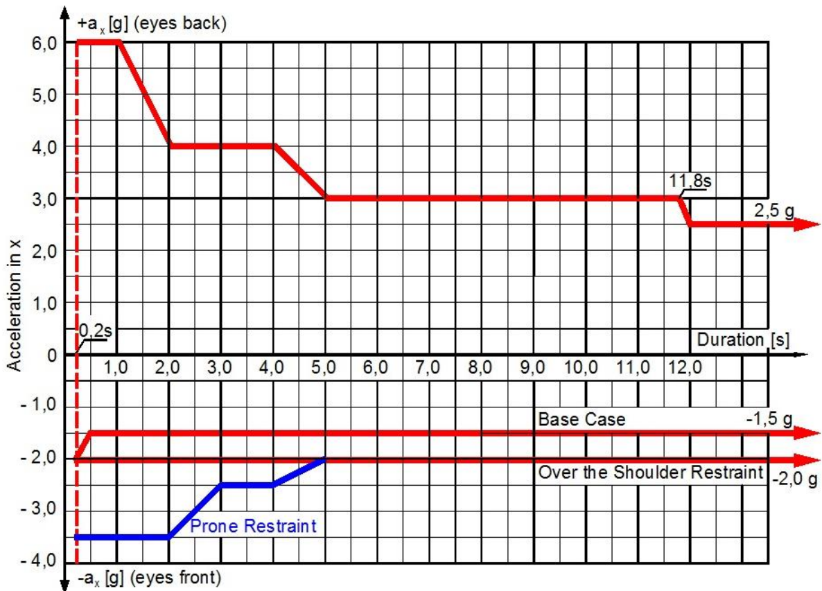
Figure 7.2 Acceleration-Duration Limits for the Acceleration in the X-Direction (Eyes Front and Eyes Back)
